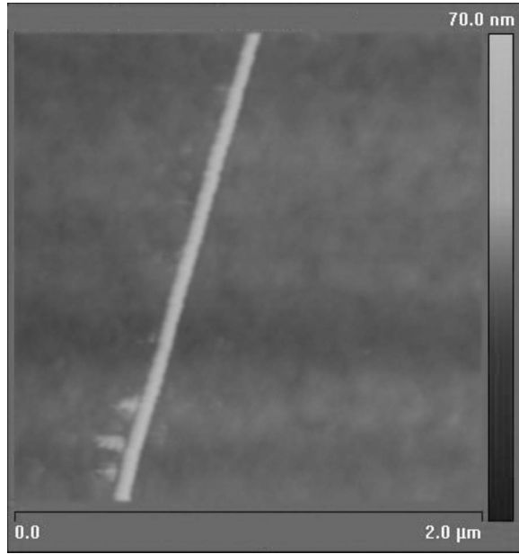
FIG. 2. AFM image of a crack in the garnet film.
